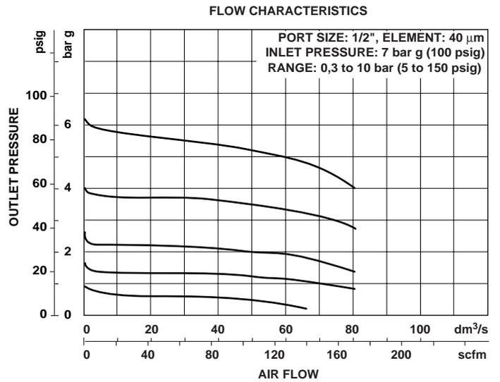
**Ordering Information.** Models listed include ISO G parallel threads, knob adjustment, automatic drain, metal bowl with liquid level indicator, 40 µm element, relieving diaphragm and 0,3 to 10 bar (5 to 150 psig) outlet pressure adjustment range\*.
