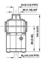
Solenoid operated plus manual shut-off with lockout
