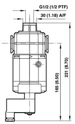
Air pilot operated plus manual shut-off with lockout
